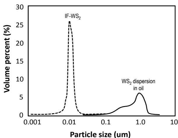
Figure 1. Particle size distributions for IF-WS<sub>2</sub> and a regular WS<sub>2</sub> dispersion in oil
