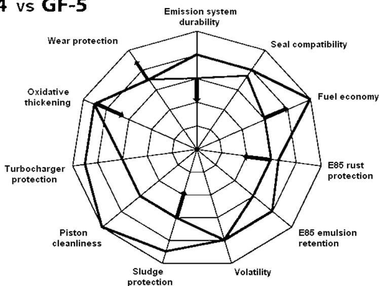
*Figure 2.* Changes in the performance spectrum of ILSAC GF-4 oil top-treated with IF-WS<sub>2</sub> emulsion
